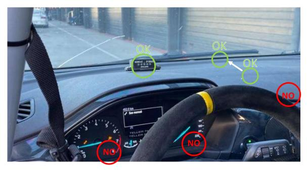
▲ **Best suggestion**: Fit the wireless *Racelink* on the dashboard (clean and dust free spot) position, in sight of the driver. If there are too many electronic devices near the *Racelink*, please position the *Racelink* closer to the window. 3M Dual Lock tape will be provided, but other mounting methods may also be used (but respect the daily recharge that is needed for the Racelink).
